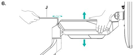
To properly balance the arm with monitors mounted, adjust the spring tension using the supplied Allen Key as follow:
