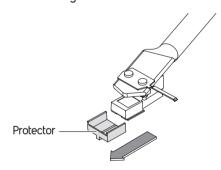
**NOTE**: Applying a downward force may cause the stylus to come off the body. Only low volume is output if the stylus has come off, or is about to come off, so refer to "Replacing the stylus" to reattach the stylus correctly.
