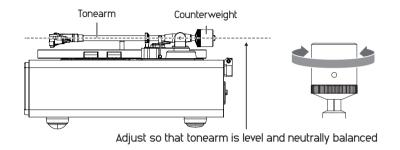
6. Once the tonearm is correctly balanced, return the tonearm to its rest and secure it in place with the clip. Hold the back of the counterweight to avoid moving its position, gently rotate the tracking force dial until the zero is in line with black center line on the rear of the tonearm. Check to make sure the tonearm is still neutrally balanced.
