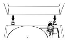
**NOTE**: It is recommended to install the lid at last to make it easier during setup and calibration.
