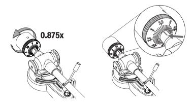
**NOTE**: Each mark on the scale represents 0.1g. The recommended tracking force for the factory-installed cartridge is 3.5g+-0.5g. Carefully rotate the tracking force dial. When "3.5" is centered over the black line on the top of the tonearm please stop.
