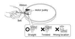
4. Finally, remove the red ribbon from the belt.
