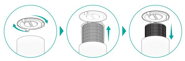
**1.** Turn the unit upside down and twist open the cover plate.
