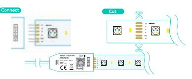
Plug the DC adapter to the LED strip lights' DC power input.
